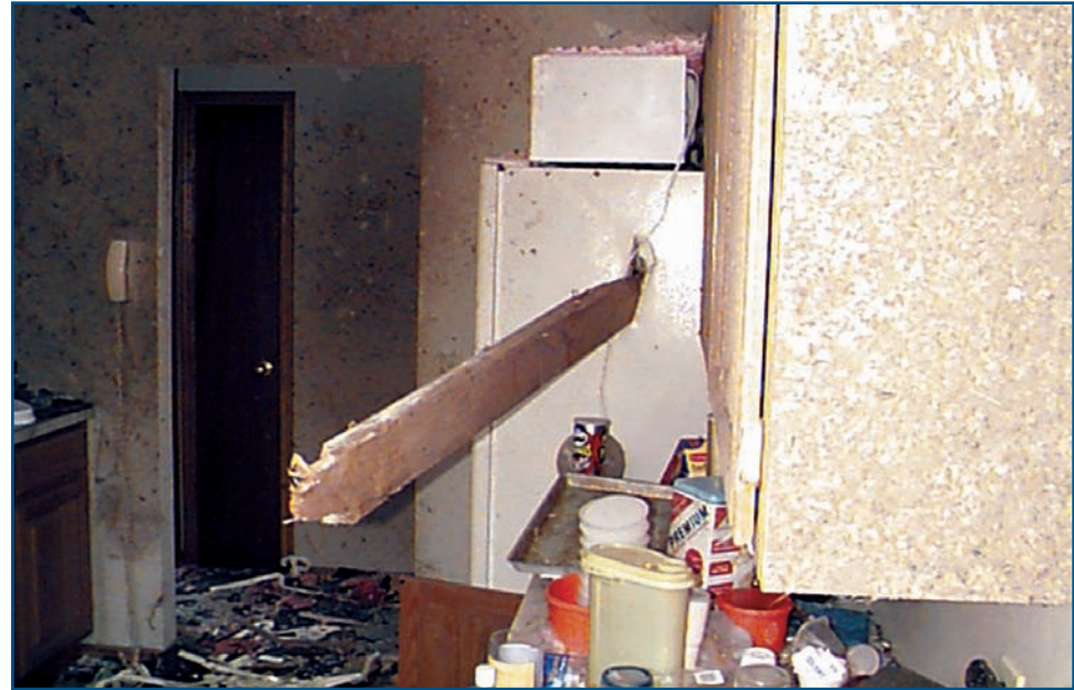
Figure 2-2 Example of damage from a windborne missile. A 2-inch by 6-inch board penetrated a refrigerator.
